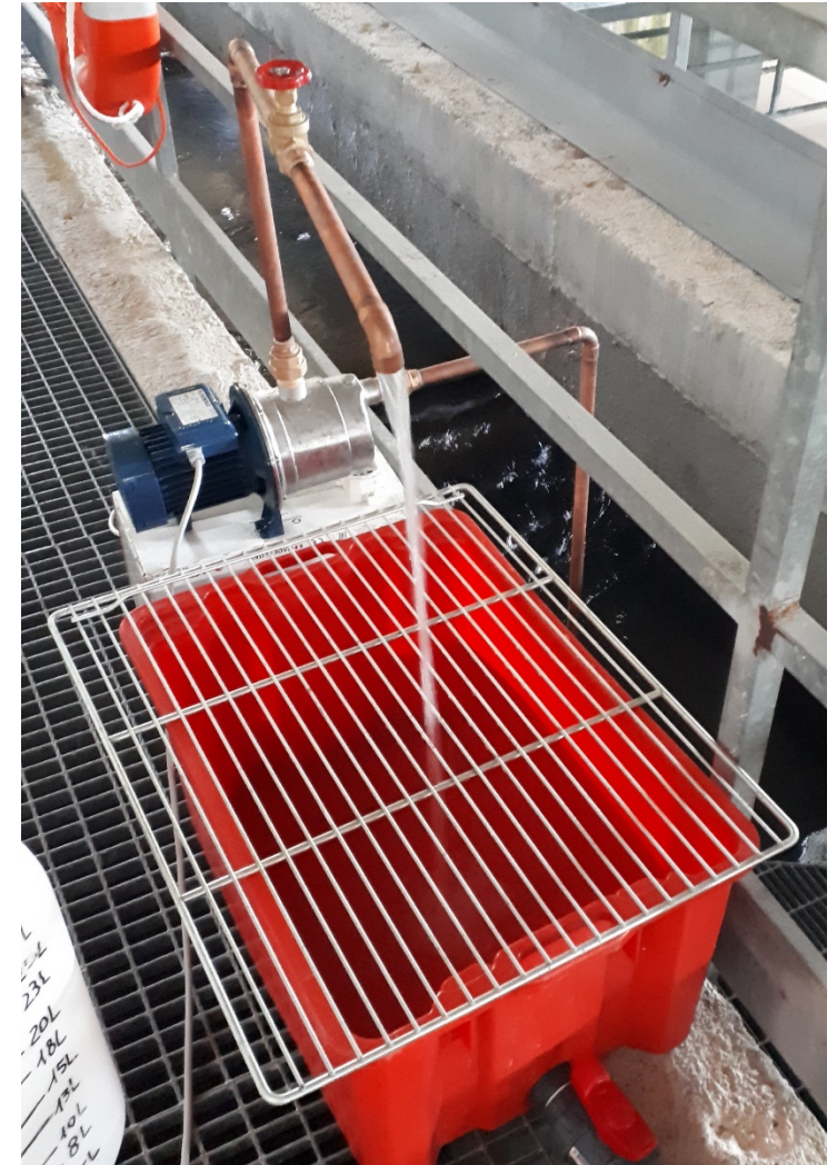
PUMPING AND SIEVING (for cases where using cartridge filter is not possible, e.g. sand filter backwash water)
