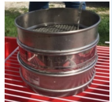
PUMPING AND SIEVING (for cases where using cartridge filter is not possible, e.g. sand filter backwash water)
