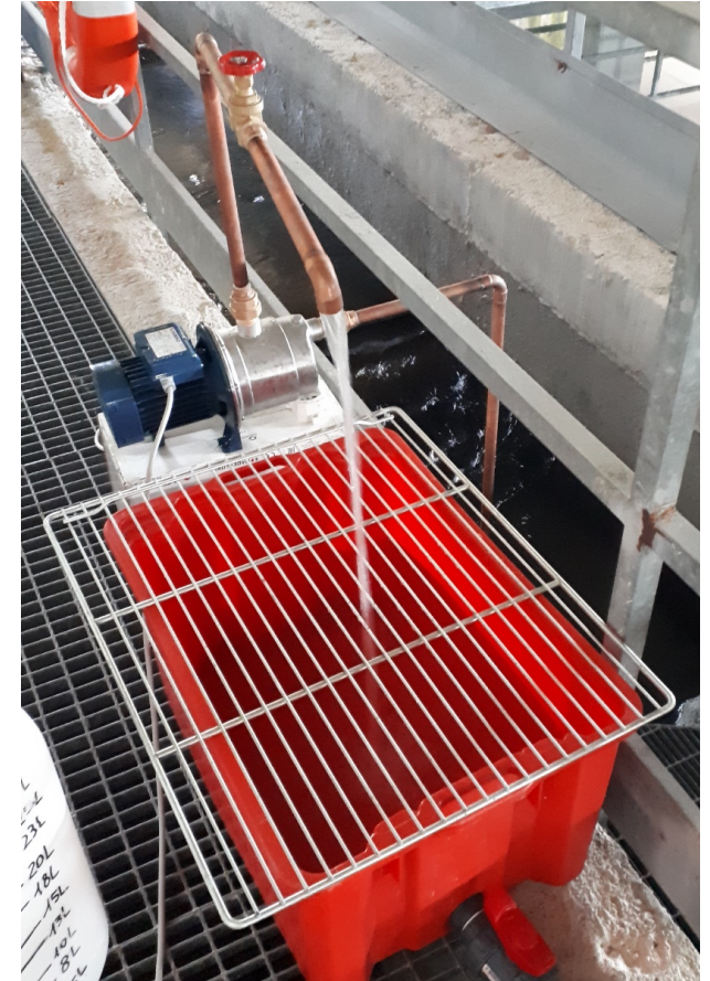
PUMPING AND SIEVING (for cases where using cartridge filter is not possible, e.g. sand filter backwash water)
